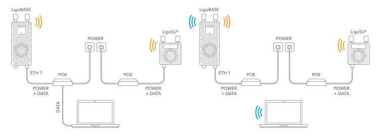
\*Multiple LigoSU units can be connected to the LigoBASE
