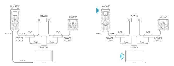
\*Multiple LigoSU units can be connected to the LigoBASE
