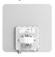
Subscriber unit with an integrated directional 23 dBi antenna.
